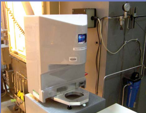
A rheometer is a device used to measure the way in which a liquid, suspension or slurry flows in response to applied forces.
