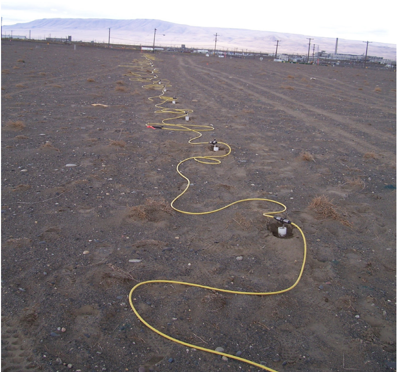
An array of electrodes is driven into the soil and connected to a central terminal where electricity is applied to measure soil resistance. The data are used to map the location, size and configuration of contaminant plumes in the vadose zone around the tanks.
