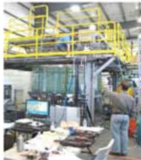
A new tank waste mixing test platform is gathering data on waste particle concentrations and distribution throughout the tank. The information will be used to decide how to accurately sample and consistently feed large batches of high-level waste to the Waste Treatment Plant.
