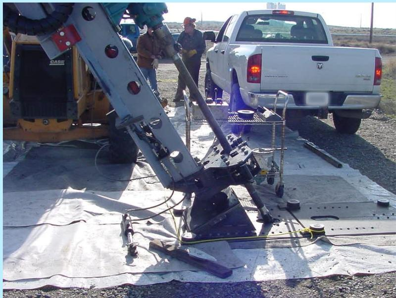
*Direct Push technology is one of the tools used by CH2M HILL to understand contaminants in the soil beneath Hanford's underground radioactive waste storage tanks. It pushes a hollow rod directly into the soil vertically or at an angle, allowing the capture of soil samples or the insertion of monitors in areas beneath structures that were previously beyond our reach. It also reduces worker exposure to contaminants and avoids bringing contaminated soil to the surface.*
